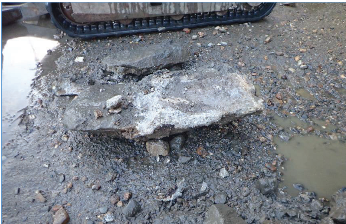
Plate 15: TP-02 showing a large stone removed from the apron. The stone measured 700mm long, 400mm wide, 100mm thick.
